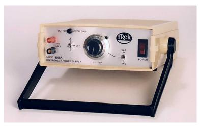
The Trek Model 605A is a high-voltage reference supply designed to provide precise control of output voltages in the range of 0 to +1 kV DC or 0 to -1 kV DC with an output current range of 0 to  $\pm 1$  mA DC.
