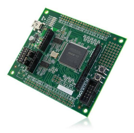
The 10M08 evaluation board will enable a cost effective entry point to MAX 10 FPGA design. The card comes complete with Arduino header socket, which will enable a wide variety of daughter cards to be connected.
