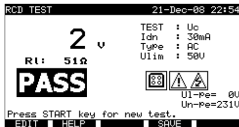
Example of contact voltage measurement results
