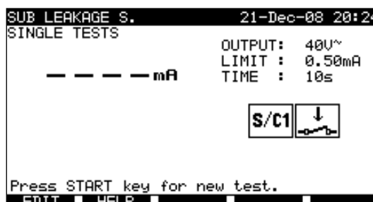
Sub leakage S menu
