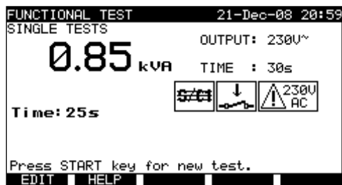
Example of apparent power measurement result
