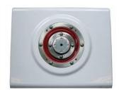
7 Place the support of the weighing plate on the balance
