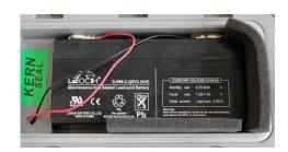
□ Insert the rechargeable battery in a manner that it cannot slip (fasten with a rubber mat)
