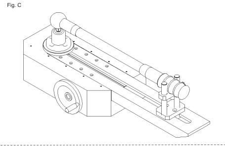
This is a typical torque wrench calibration application.
