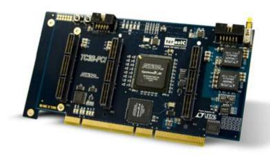
The TERASIC Cyclone® III PCI-X development board provides a hardware platform for developing and prototyping low-power, high-performance, logic-intensive PCI-based designs. The board has a high-density of the external memory to facilitate the design and development of FPGA designs which need huge storage capacity and high bandwidth memory. It also includes Low-Voltage Differential Signaling (LVDS) interface of the High-Speed Terasic Connectors (HSTCs) for extra high-speed interface application.
