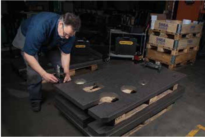
Flatness measurement of machine end after machining.
