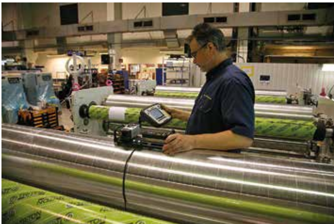
Checking roll parallelism using the Easy-Laser Roll alignment kit.
