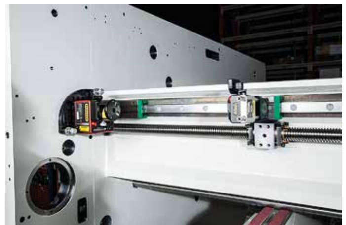
Straightness measurement of linear guide with laser transmitter D22 from system E720.
