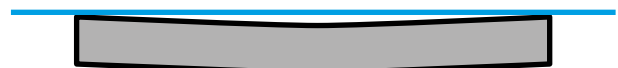
The linear guides can be parallel, but both beams may be crooked at the same place.
