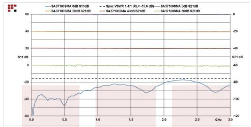
0 to 100 dB Step Attenuator With a 1 dB Step SMA Female Connectors Rated Up To 3 GHz and Up to 2 Watts in a Dial Design from Fairview Microwave is in-stock and available to ship same-day. All of our RF/microwave products are available off-the-shelf from our ISO 9001:2008 certified facilities in Allen, Texas. Fairview Microwave is RF on-demand.
