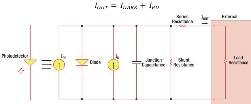
Figure 1 Photodiode Model
