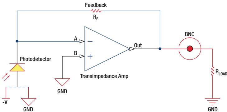
**Figure 3 Amplified Detector**
