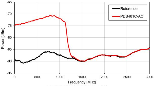
PDB481C-AC - Typical RF-OUTPUT Spectral Noise
