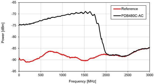
PDB480C-AC - Typical RF-OUTPUT Spectral Noise
