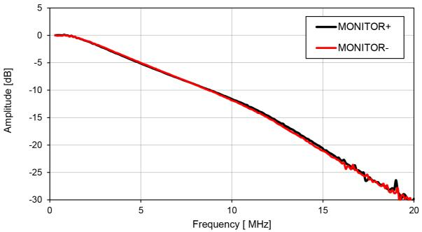
PDB481C-AC - Typical MONITOR OUTPUT Frequency Response
