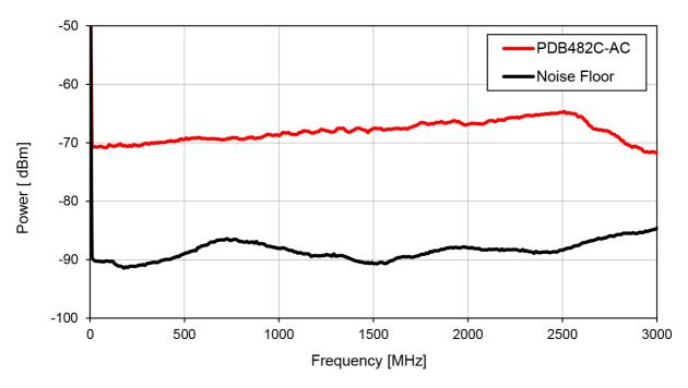
PDB482C-AC - Typical RF-OUTPUT Spectral Noise
