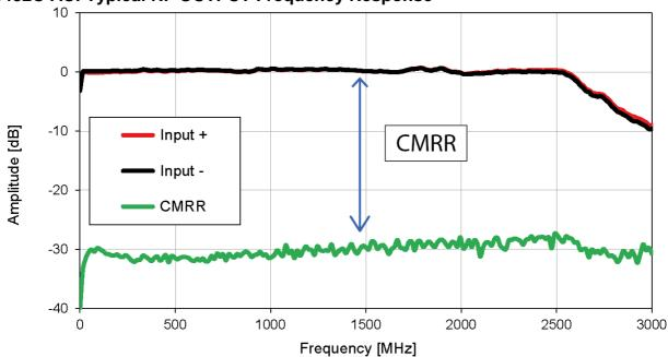
PDB482C-AC - Typical RF OUTPUT Frequency Response
