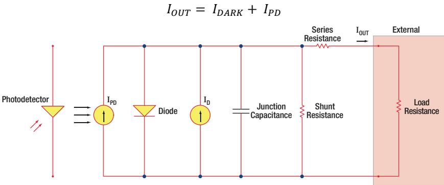
Figure 1 Photodiode Model
