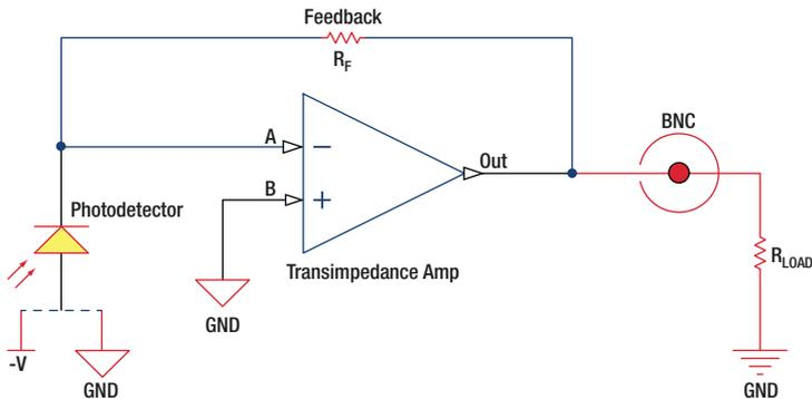
**Figure 3 Amplified Detector**
