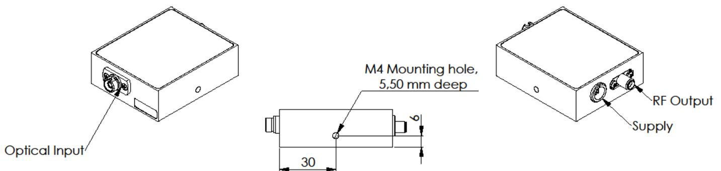
Dimensional unit is millimeter [mm].
