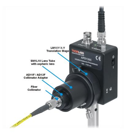
The assembly in front of the APD130x comprises of a fiber collimator (dependent on fiber), a lens tube collimator adapter (AD11F or AD12F, dependent on collimator), a SM1L1 lens tube with aspheric lens inside (not visible above) and a LM1XY X-Y translation mount.
