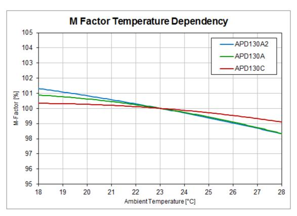
Typical Dependency of the M Factor vs. Temperature - APD130x
