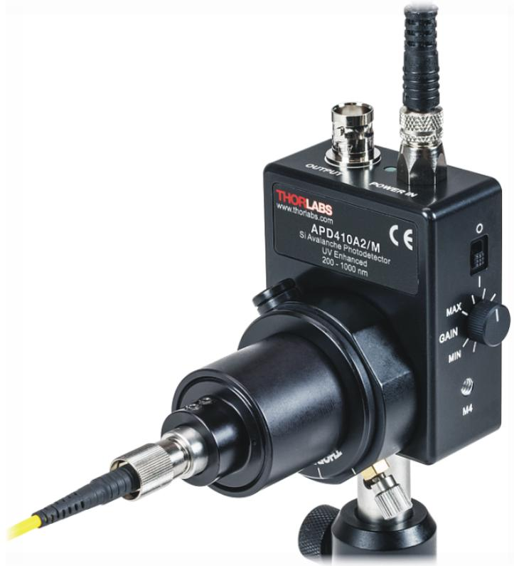
The assembly in front of the APD410x comprises of a fiber collimator (dependent on fiber), a lens tube collimator adapter (AD11F or AD12F, dependent on collimator), a SM1L1 lens tube with aspheric lens inside (not visible above) and a LM1XY X-Y translation mount.
