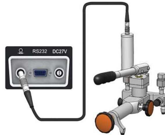
Figure 3-11 External pressure module
