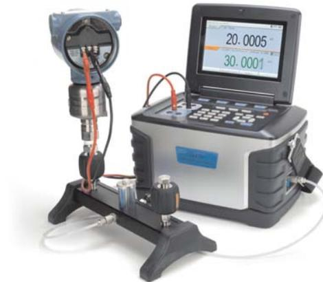
Figure 3-3 Gauge pressure source
