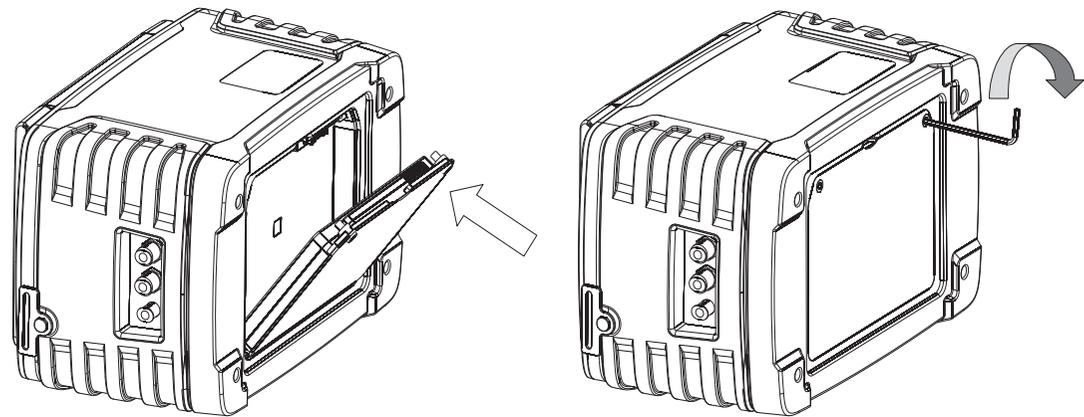
Figure 2-4 Battery installation
