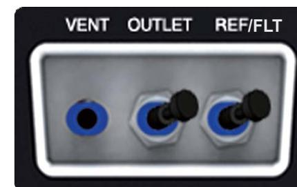
Figure 2-6 Pneumatic connection
