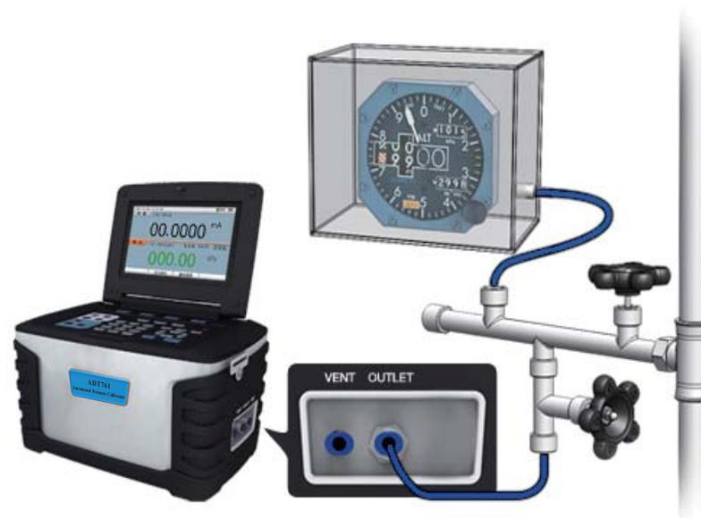
Figure 5-4 Calibrating a barometer altimeter
