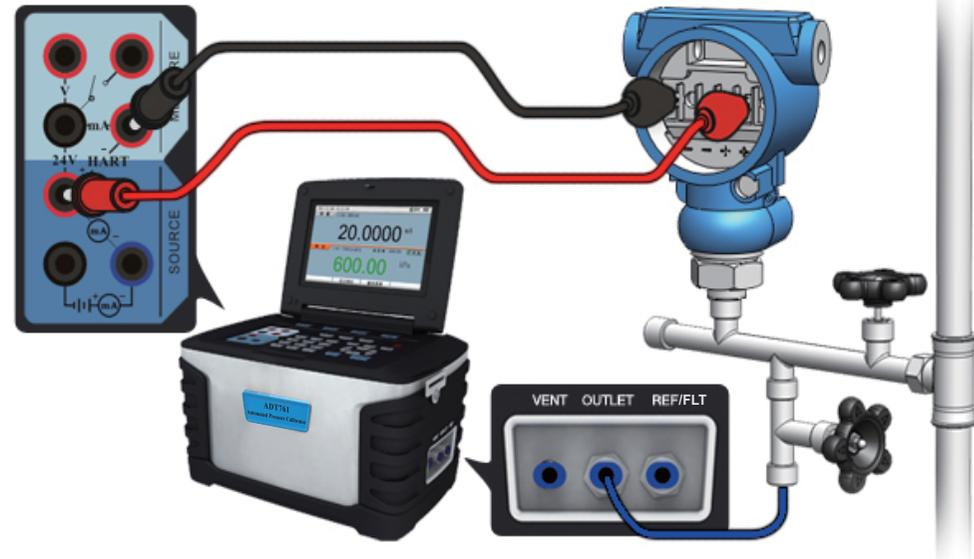
Figure 3-17 Calibrating a pressure transmitter
