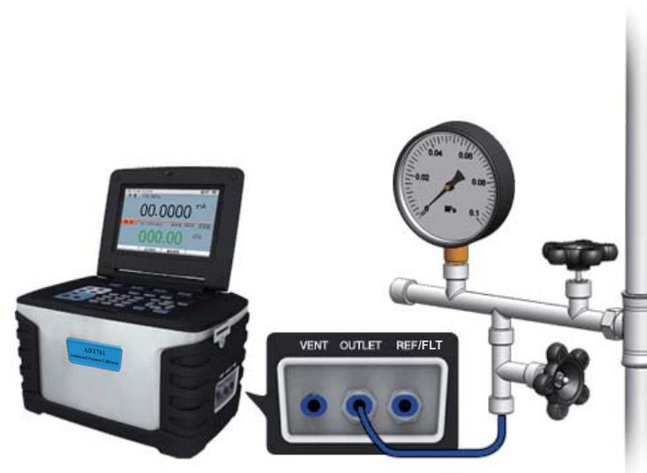
Figure 3-20 Calibrating a dial pressure gauge
