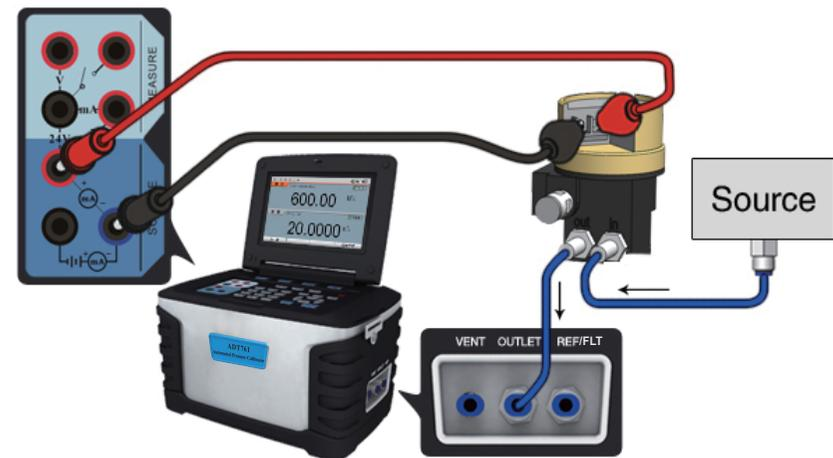
Figure 3-24 Calibrating an I/P converter
