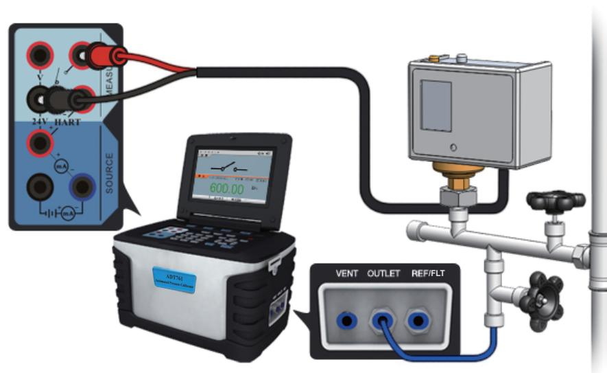
Figure 3-18 Calibrating a pressure switch
