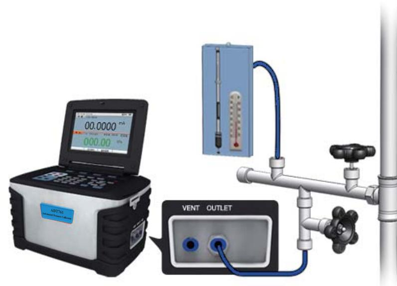
Figure 5-2 Calibrating a mercurial barometer
