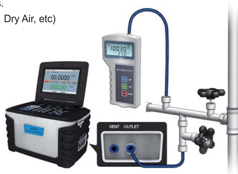
Figure 5-1 Calibrating a digital barometer
