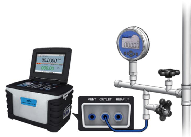
Figure 3-21 Calibrating a digital pressure gauge
