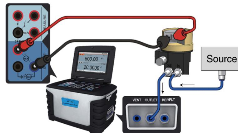
Figure 3-19 Calibrating a I/P converter
