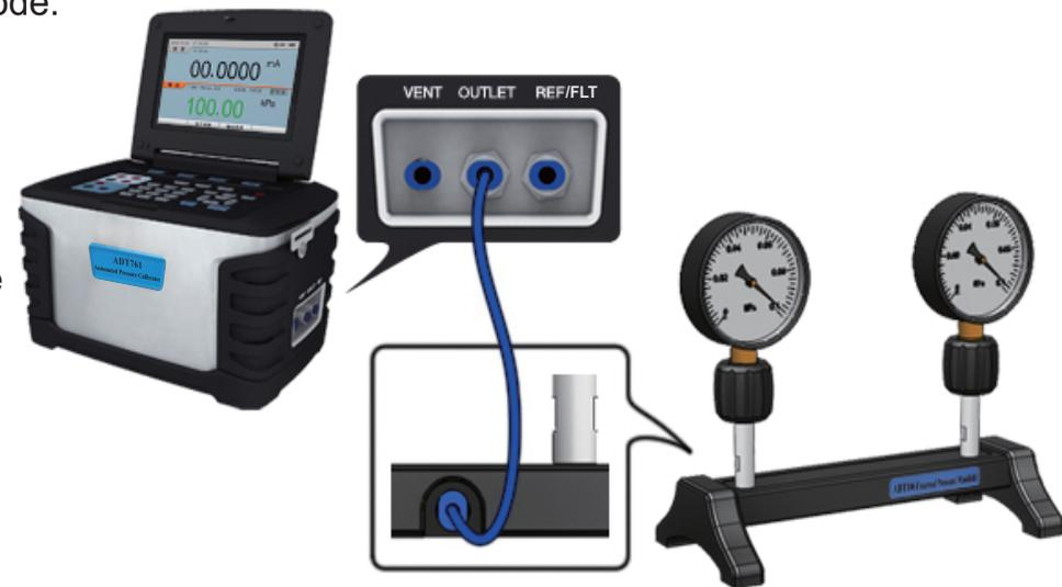
Figure 3-16 Calibrating pressure gauges
