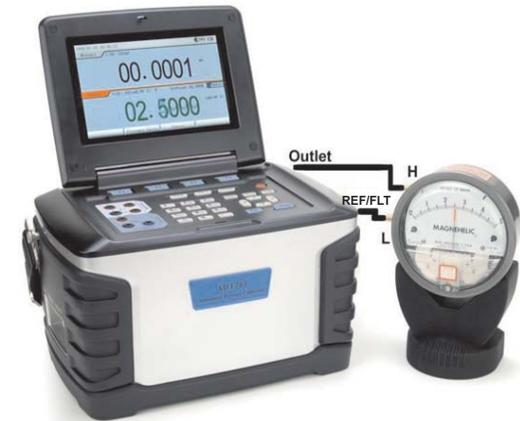
Figure 3-4 Differential pressure source
