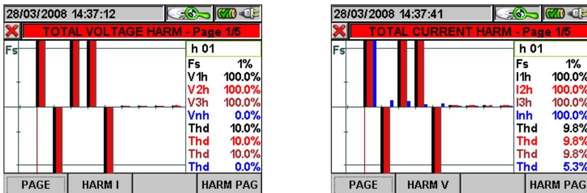
Fig. 146: Total harmonics in three-phase 4-wire system
