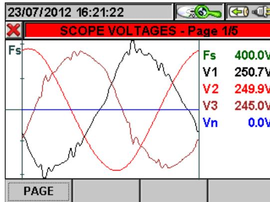
Fig. 145: Voltage scope in three-phase 4-wire system
