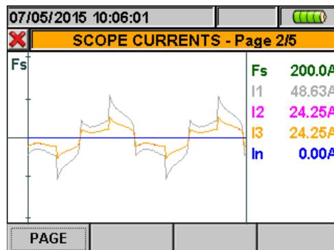
Fig. 37: Current waveforms screen for 4-wire systems
