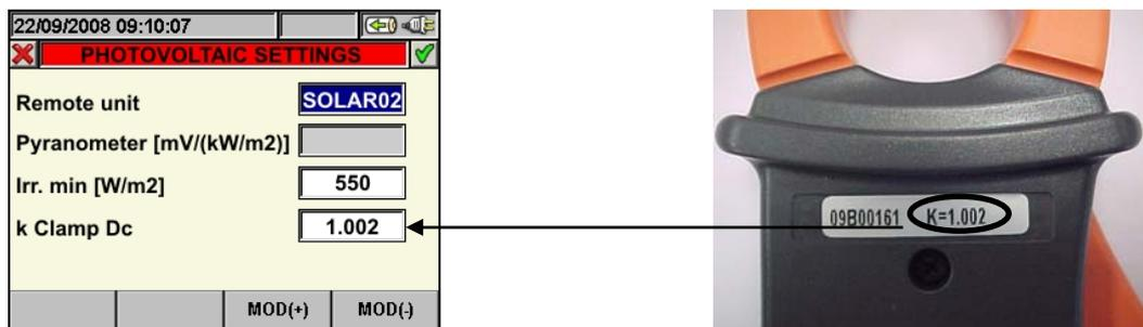
Fig. 67: Set of corrective constant for DC clamp
