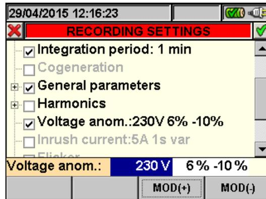
Fig. 90: Voltage Anomalies screen - setting control parameters
