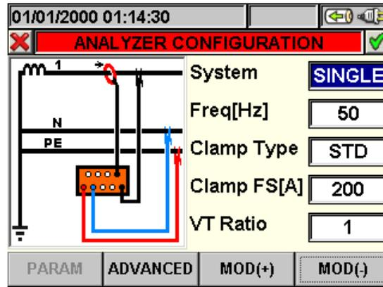
Fig. 59: Analyzer Configuration screen for SINGLE phase system
