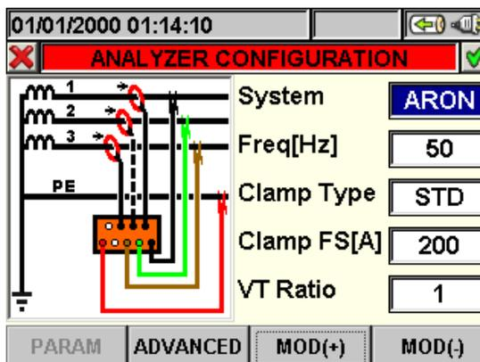
Fig. 58: Analyzer Configuration screen for ARON system
