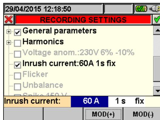
Fig. 92: Inrush current screen - setting control parameters
