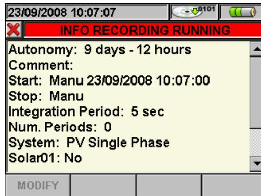
Fig. 103: Screen with information about recording in progress with PV system set
