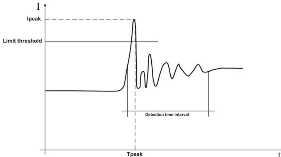
Fig. 175: Parameters of oscillating inrush current event
