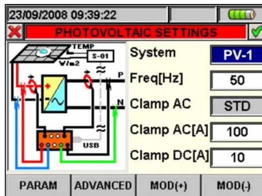
Fig. 52: Screen for analyzer configuration for PV-1 system
