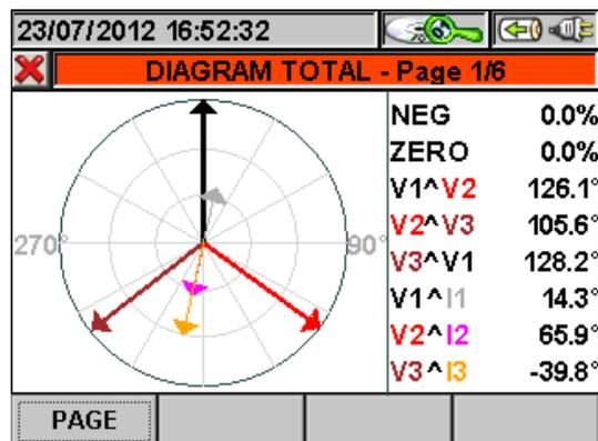
Fig. 147: Total vector diagram in three-phase 4-wire system
