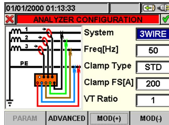
Fig. 57: Analyzer Configuration screen for 3-wire system
