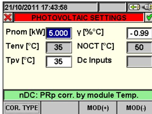
Fig. 65: Parameter setting screen for PV systems
