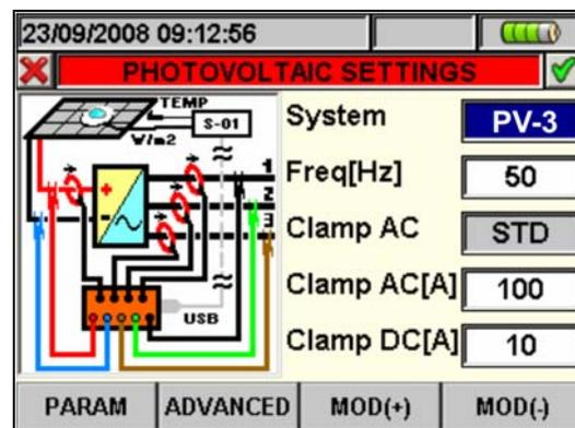
Fig. 53: Screen for analyzer configuration for PV-3 system
