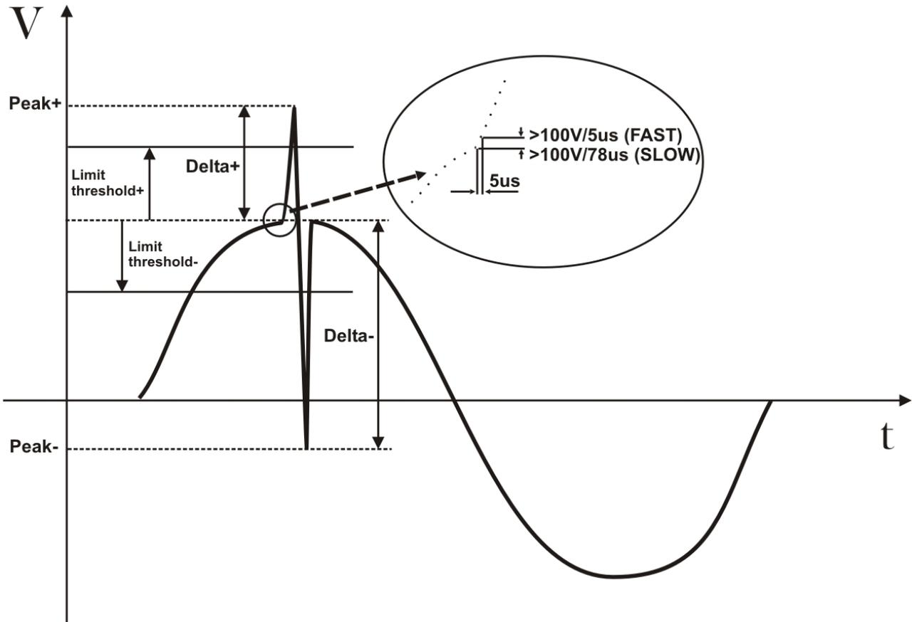
Fig. 177: Typical voltage spikes at 50Hz frequency
