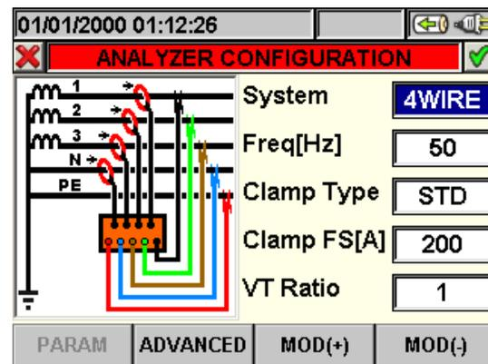
Fig. 56: Analyzer configuration screen for 4-wire system
