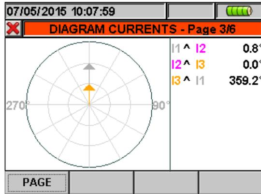
Fig. 49: Vectorial current diagram for 4-wire system
