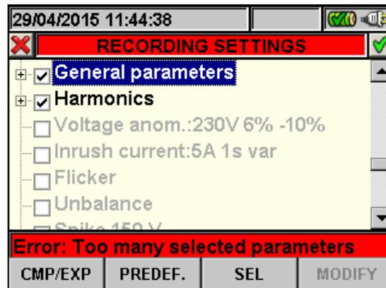
Fig. 83: General Parameters section: too many selected parameters
