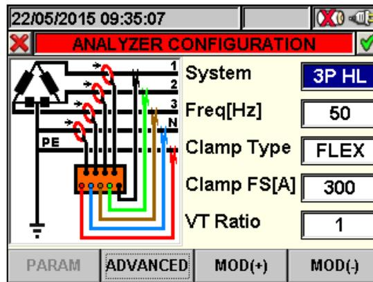
Fig. 63: Analyzer Configuration screen for Three phase system 4-wire 3P HL
