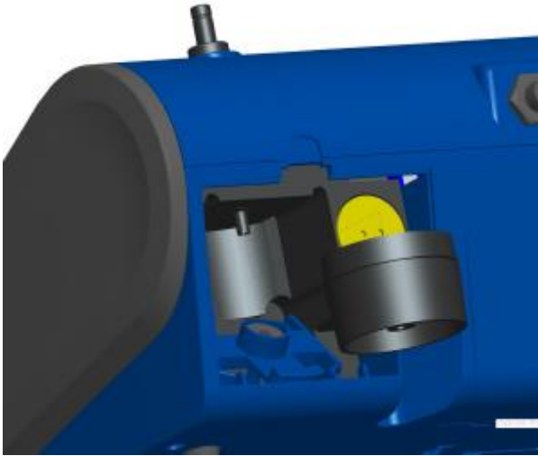
Figure 4-8: Remove 37-mm Filter Cassette
