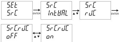
1 Simultaneously press the CLEAR and ENTER keys to switch to setting mode.
