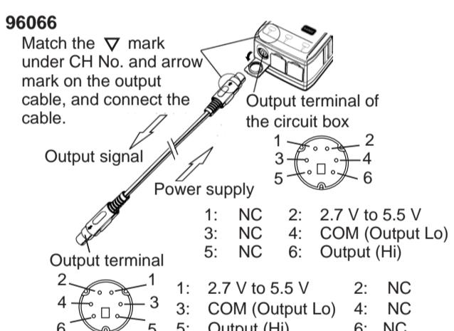
\* This instrument is supplied power via an output cable. Power supply of 2.7 to 5.5 V (200 mVA) is required between 1 and 3 of the output terminal and between 2 and 4 of the output connector.
