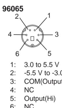
\* This clamp-on probe is supplied power via an output cable. Power supply of +3.0 to +5.5 V is required between 1 and 3 of the output terminal and -3.0 to -5.5 V is required between 2 and 3 of the output terminal.
