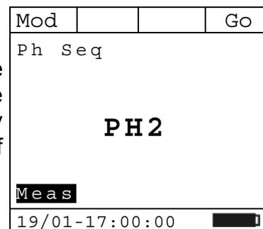
7. If there is concordance between the two phases, to which the test lead has been connected, the instrument displays the screen here to the side. Otherwise, it displays “**123**” or “**132**”.
