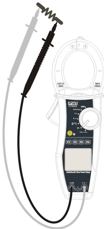
Fig. 13: resistance measurement
