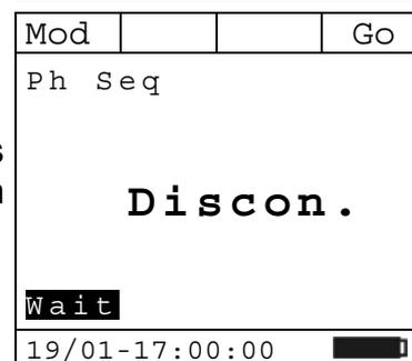
5. The instrument shows the screen here to the side, and waits for the detection of the second sequence of phase L1. Connect the test lead to phase L1 of the second sequence.
