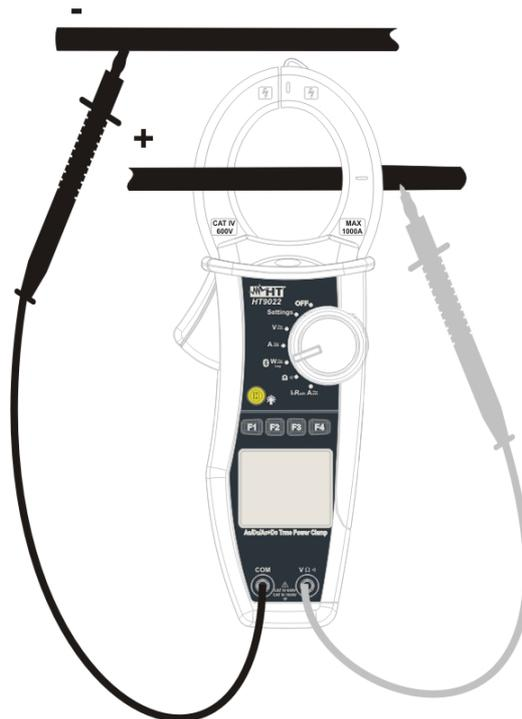
Fig. 11: DC power measurement
