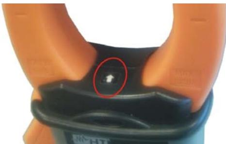
The photo in Fig. 4: current direction arrow shows an arrow which indicates the conventional direction of current.
