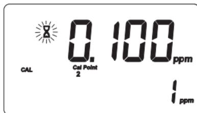
**Note:** The instrument will automatically skip the standard value used for the first point.
