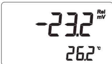
**Note:** Press the right or left arrow key to toggle between temperature and absolute mV reading on the secondary LCD.
