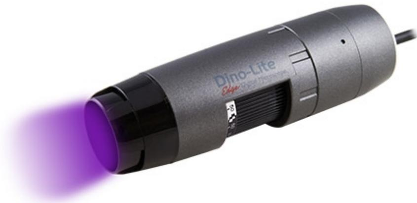
The AM4115TW-GFBW Dino-Lite Edge series digital microscope features superior optics, a macro zoom design, and 480nm (blue) excitation light with a 510nm emission filter for observing green fluorescence in life-size objects, such as biological samples (e.g. mice, leaves, zebra fish).
