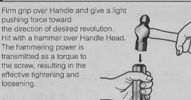
Remark: Hammering with more force than necessary may cause distortion or malfunction of the product.
