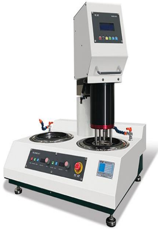
KPM-203D-AH32 / Polishing Machine / Preparing Specimens
