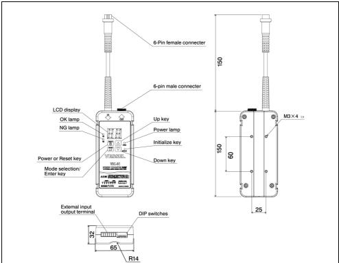
\*1: The substrate can be damaged if fixed with a screw that is 12mm or longer.
