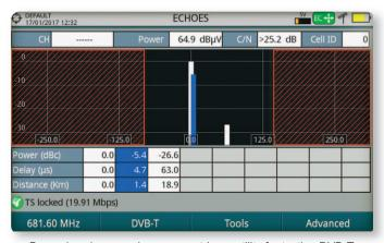
Dynamic echoes analyzer, a must-have utility for testing DVB-T, DVB-T2 and DVB-C2 networks.
