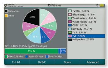
The bitrate analysis shows on a pie chart the real-time bitrate used by each one of the services in a transport stream.
