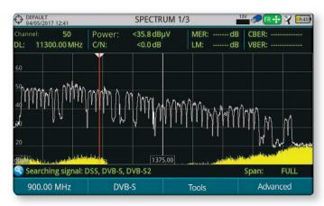
Freeze the spectrum graph and compare it with the running trace. Save that information and use it to identify satellites based on their spectrum footprint.
