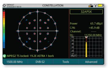
The fastest way to identify signal impairments. There are different types of constellation diagrams for the different modulation modes.
