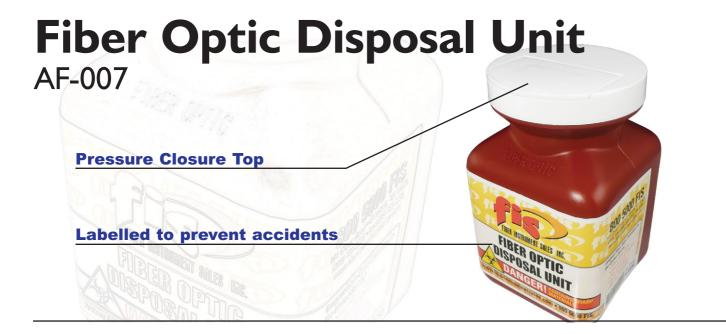
A practical and simple way to dispose tips from cut fibers. Perfect to use on-site. The top has a snap closure to avoid discarded fiber tips out from the disposal. The disposal is labelled to avoid accidents with the sharp tips of optical fibers contained in.
