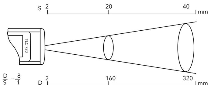
Please ensure that the object being measured is larger than the distance between the two laser points. The smaller the measured object is, the closer you must be to the object.
