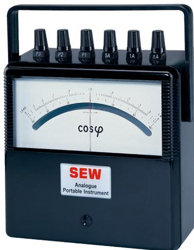
The PF meter is used for measurement in single-phase and balanced three-phase circuits. From a phase discriminating circuits, the output of the built-in transducer produces a DC proportional to the phase between voltage and current to operate the DC indicator.
