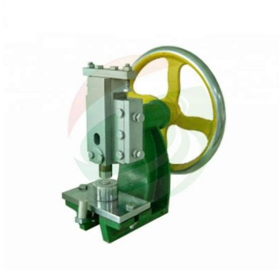
The crimper is suitable for sealing various types of coin cells such as CR2032, CR2025, and CR2016 with adjust the sealing height and with out changing the die.
