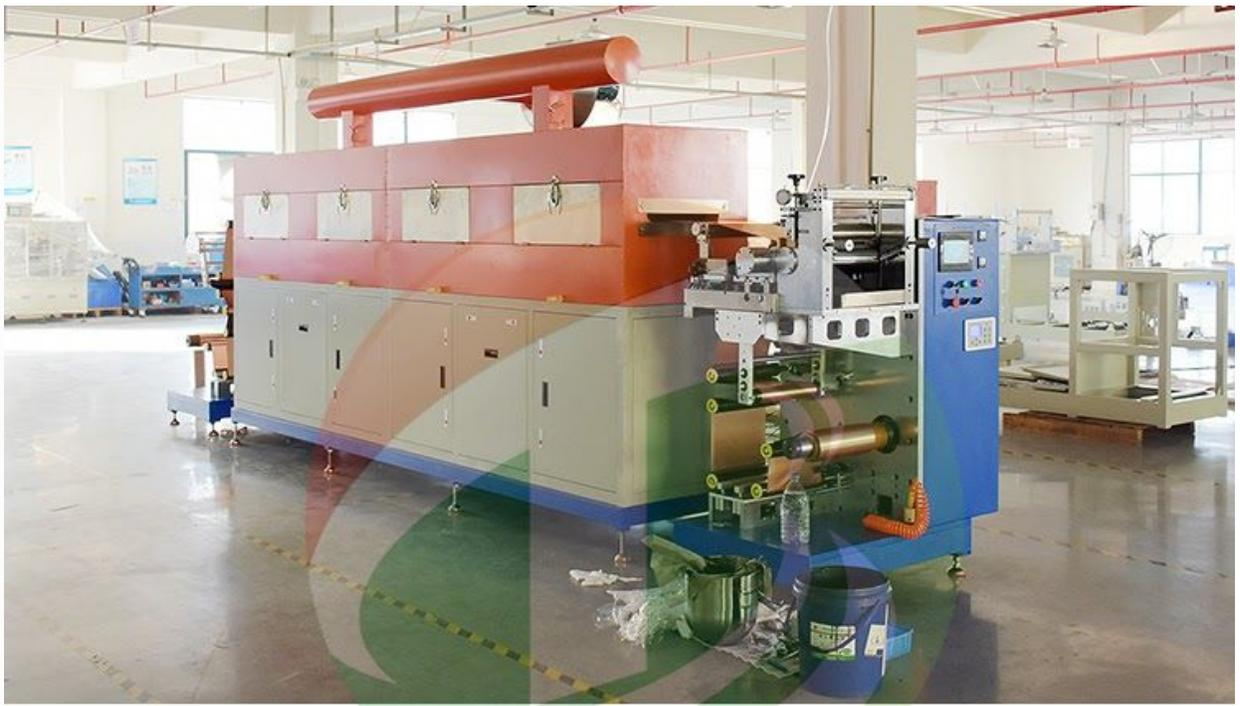
Pour in battery slurry ⇒ Coating ⇒ Drying process ⇒ Winding
