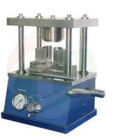
TOB-MSK-510M is a compact hydraulic crimper for sealing all types of cylinder cases in battery R&D labs. The compact body design allows it to be easily placed inside a glove box and thus preventing contamination of the electrolyte materials during cell assembly. Simple operation with safety protection feature allows customers to master the sealing procedure within 5 minutes.
