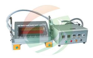
TOB-YF350-S compact vacuum sealing machine is mainly used for sealing aluminum-laminated case in glove box after injection of electrolyte into pouch Li-ion cell or after formation for final seal (polymer Li-lon cell). Heatable sealer blade is built into the chamber, automatically sealing the aluminum film pouch case for polymer battery.
