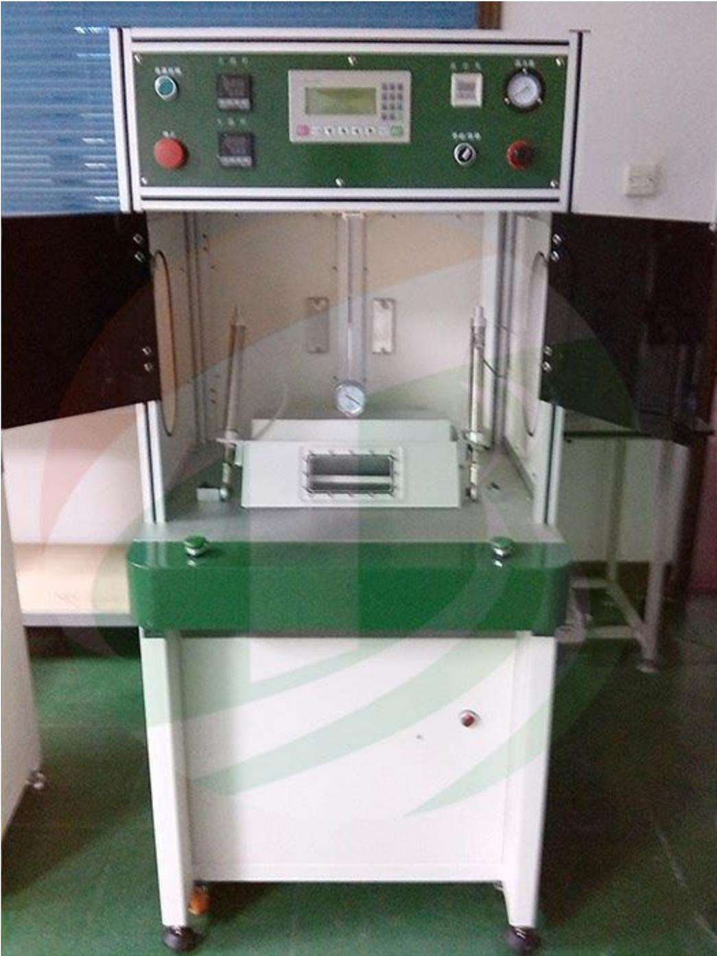
**Vacuum sealing machine sealing head**
