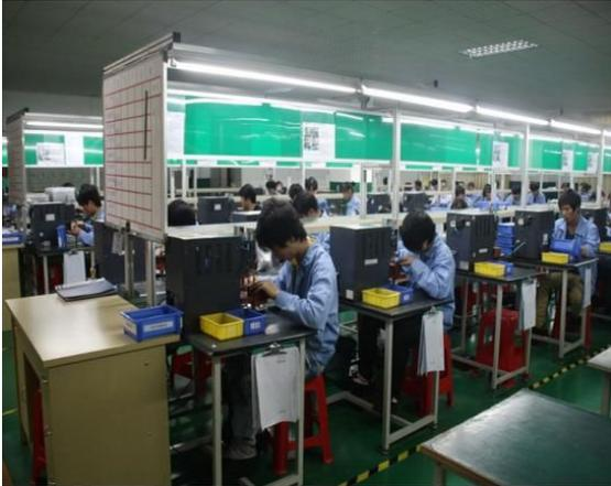
It is a manual battery production line for lithium-ion pouch cell manufacturing.
