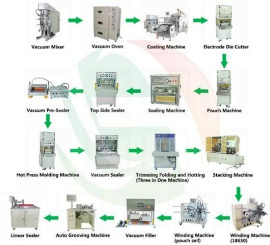
TOB offers the most professional battery and supercapacitor pilot line equipment for battery research and manufacturing.
