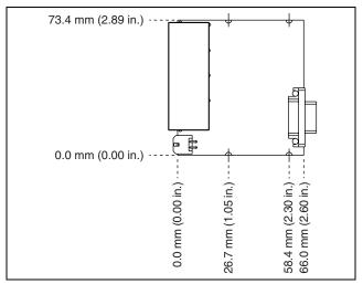
Figure 1. NI 9871E Dimensions in Millimeters (Inches)
