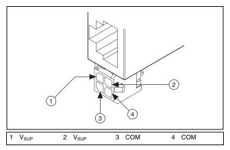
Figure 2. Four-Position External Power Connector
