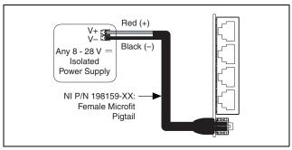
Figure 3. Powering the NI 9871E from an Isolated Power Source
