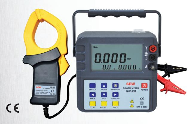
Monitor the efficiency of your appliances and equipment, and reduce your power bill with the new power meter 2015 PM.
