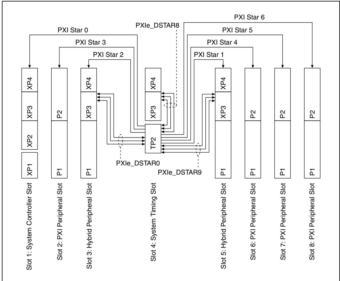
**Figure 1-3.** PXIe\_DSTAR and PXI Star Connectivity Diagram
