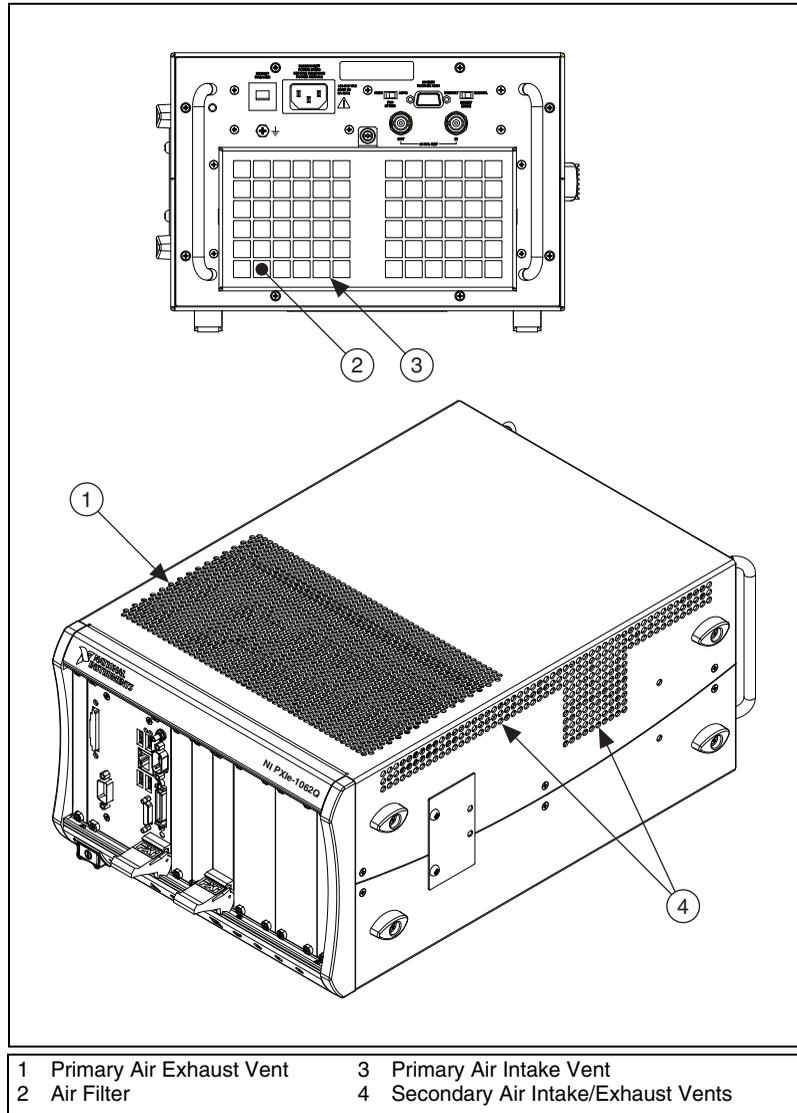
Figure 2-2. NI PXIe-1062Q Vents
