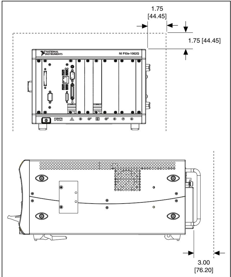
Figure 2-1. NI PXIe-1062Q Cooling Clearances
