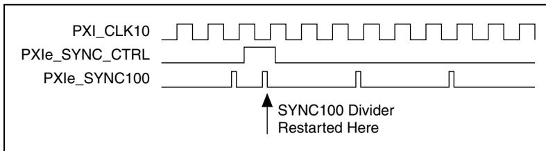
**Figure 1-7.** PXIe\_SYNC100 at 3.33 MHz Using PXIe\_SYNC\_CTRL as Restart
