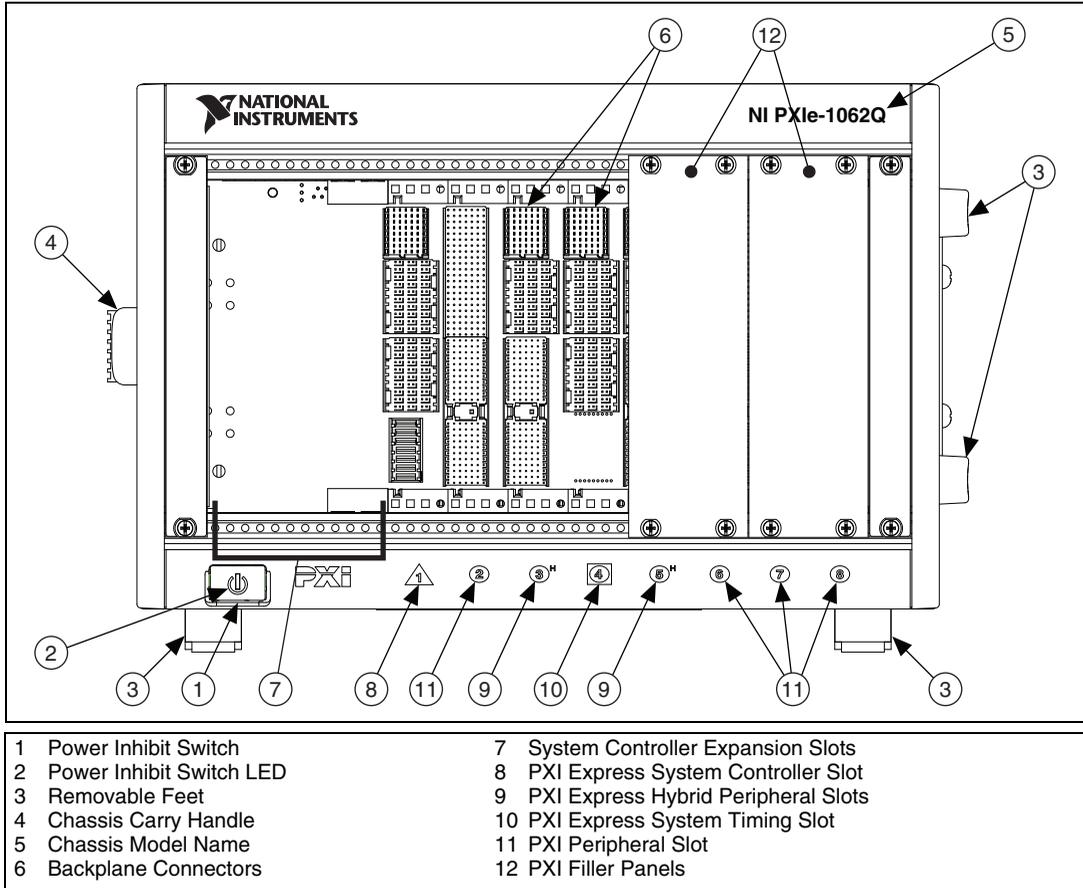
**Figure 1-1.** Front View of the NI PXIe-1062Q Chassis
