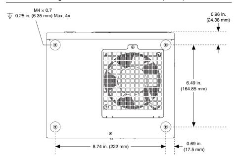
Figure 5. PXIe-1073 Chassis Rack Mount Kit Components
